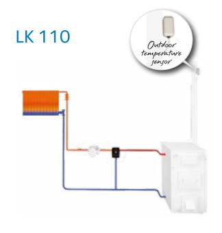
Electronic weather compensated temperature controller for hydronic radiator and underfloor heating systems.
