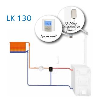
Electronic, weather compensated, indoor temperature controller for hydronic radiator and underfloor heating systems.
