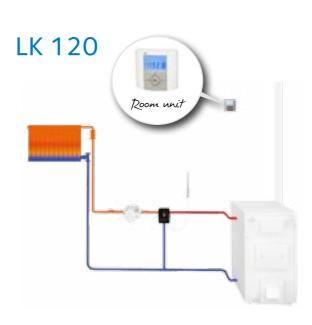
Electronic indoor temperature controller for hydronic radiator and underfloor heating systems.
