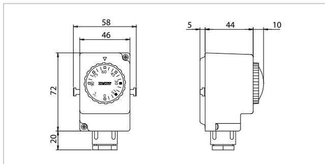
TCR is a liquid expansion boxed thermostat, unipolar, with interrupted or changeover switches, for contact appliances. Particularly suitable for measuring and regulating temperature.
