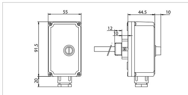
LSC1 is a boxed immersion thermostat, with liquid expansion probe, unipolar, safety temperature limiter with manual reset, fail-safe for capillary breakage, complete with watertight protection pocket. Useful in appliances where safety is required due to the temperature increase.
