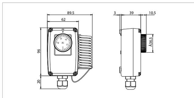
ERT/TA is an adjustable boxed thermostat for controlling the temperature in various appliances, particularly suitable for environments with a high degree of pollution.
