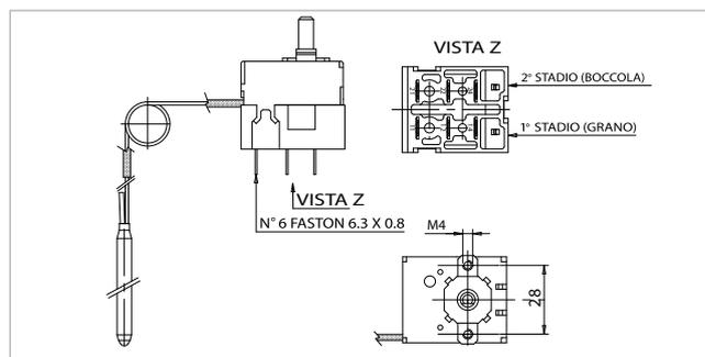
TRZ is a capillary thermostat with liquid expansion probe and 2-stage switch, unipolar, with switching contacts, particularly suitable for automatic temperature regulation for applications in civil and industrial heating, air conditioning and household appliances such as radiators electric, boilers, washing machines, dish-washers, etc.
