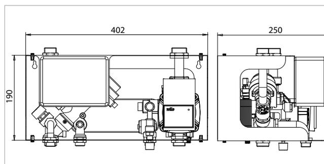
WATERWARM is a compact hydraulic kit, combined with a pellet stove or a thermo-fireplace, which allows the production of domestic hot water and water for heating. It includes a delivery/return group, a brazed exchanger with 20 plates, a diverter valve, a flow switch, an ErP circulator with degasser and built-in drain (only for code 561551) and a pre-wired electrical junction box. Includes white painted cover casing.
