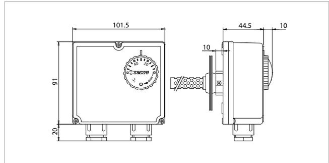
TTCA is a double regulation thermostat for burner control (internal regulation) and fan start or stop (external regulation).
