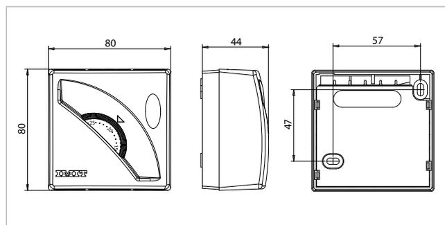
TA3 is a mechanical wall thermostat with saturated steam expansion tank, ideal for regulating home or office temperature. It is available in LED versions, without LED, ON / OFF (to turn off the thermostat without turning the knob), Summer / Winter (to connect and regulate the air conditioning or heating system). This thermostat also offers the possibility to limit or block the set temperature, through the installation of an optional switch under the cover.
