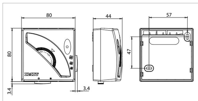
FAN TA3 SE is an electromechanical steam expansion regulator for fan-coils, radiators and fan convectors. It is ideal for regulating home or office temperature in its two modes of operation: Summer/Winter (to activate the air conditioning or heating functions). It is also equipped with a mechanical three-position switch for regulating fan speeds and to control the hot/cold valve.
