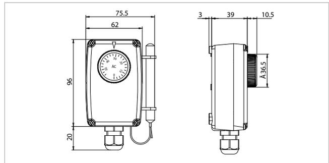
ETR is an adjustable boxed thermostat for controlling temperature in various appliances, especially suitable for environments with a high degree of pollution. Protection rating IP54.
