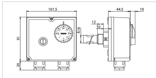
TLSC is a double boxed immersion thermostat, with liquid expansion probes, unipolar, temperature regulator and temperature limiter, fail-safe for capillary breakage, complete with watertight protection pocket. Particularly suitable for appliances where temperature control and safety is required.
