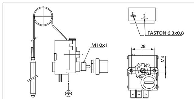
LS1 / LS3 is a capillary thermostat with a liquid expansion probe, unipolar, with safety temperature limiter with manual or automatic reset and with positive safety in case of capillary breakage. It is particularly suitable for boilers, heating systems and in all those appliances where it is necessary not to exceed a maximum set temperature.
