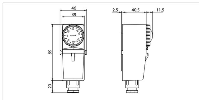
BRC is a bimetallic boxed thermostat, unipolar, with interrupted or changeover switches. Especially suitable for measuring and regulating temperature
