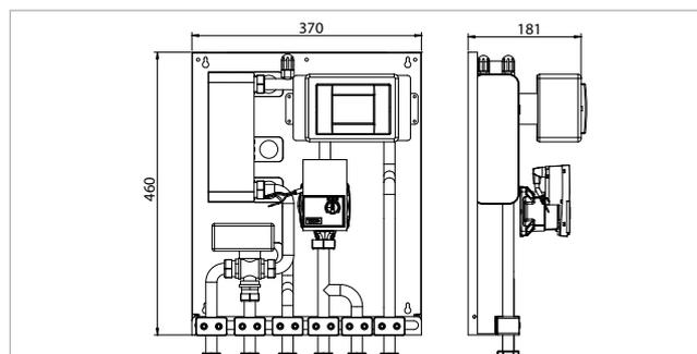
WATERLINK WTL6 is a hydraulic separation module between two heat generators powered by different energy sources. The most typical appliance is that between a thermo-fireplace (or a thermo-heater) and a gas boiler. When handling heat produced by the biomass source, the module disables the traditional boiler and activates the 3-way valve to send hot water to the domestic heating system. Otherwise the 3-way valve is not enabled, allowing the gas boiler to meet the required heating needs.
