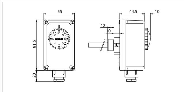
TC2 is a boxed immersion thermostat with liquid expansion, unipolar, with changeover switches, complete with a watertight protection pocket. The thermostat normally applied on delivery piping is particularly suitable for the automatic regulation of boilers, pumps and other various appliances. It is also available in a capillary version.
