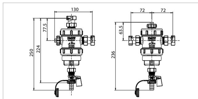
STORM is a cyclonic technology magnetic dirt separator with double magnet. Thanks to its 2 separation chambers, it retains all ferrous and non-ferrous particles that are harmful to the domestic boiler. May be installed as a part of a unit or directly, complete with fixing nozzles and dirt drain tap.
