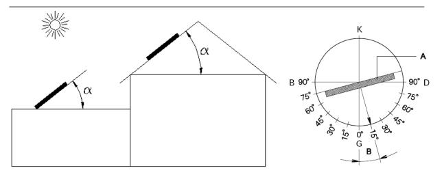
A- Collector deflection B- Azimut Angle
